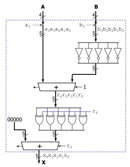
The figure below depicts the internal architecture of the 4-bit adder and the 5-bit adder. The full adder (FA) circuit is also shown.
